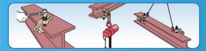
This screw clamp can be used for a variety of operations such as lifting up and down, lateral (horizontal) pulling and turning over. Adequacy of tightening can be visually confirmed by secure and safety structure.
