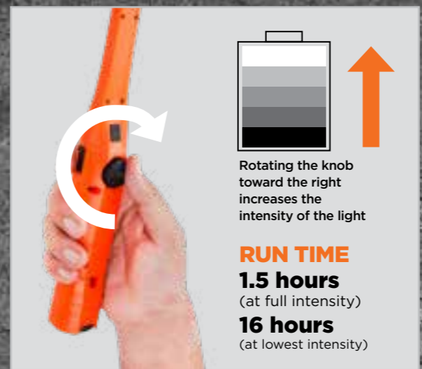
Adjust the light intensity via simple to use rotating knob
