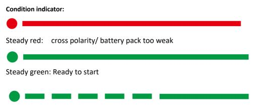
Green blinking for 5 second then steady: Bypass mode
