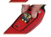
Position the new Circuit Breaker into the housing, take care to line up the breaker spades with the breaker terminals, and press down gently until the Circuit Breaker is fully engaged into the breaker terminals. Replace the rear cover and the two retaining screws.
