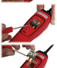
Using an appropriate pry tool or small screwdriver, carefully pry the Circuit Breaker towards the tip to dis-engage it from the breaker terminals. Do not apply excessive force.
