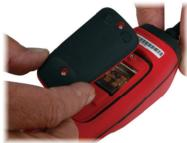
Unscrew the two retaining screws and remove the rear cover.
