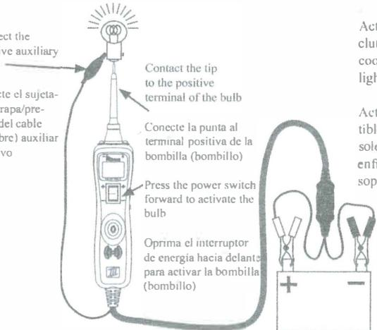
Activate fuel pumps, magnetic clutches, starter solenoids, cooling fans, blower motors, lights etc.
