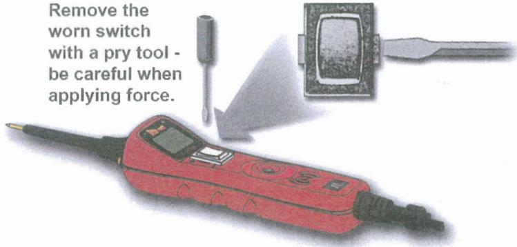
Make sure to install the switch straight and press until flush with casing.
