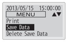
②Confirmation screen as shown in the right is displayed. Select "YES" and press ← (ENTER) Key for saving the test result. Select "NO" and press ← (ENTER) Key for go back to Menu screen (previous Step ①).
