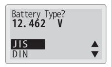
Press **⇒** (BACK) Key to go back to the Battery Voltage Selection screen (Step ③).
