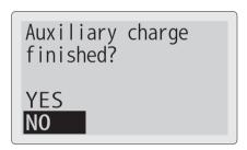
\*\*Select "YES" when the test result is "Charge/Retest", the test result changes "Replace".
