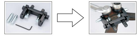
• Designed for twin ball joints as fitted to Audi and VW control arms.
