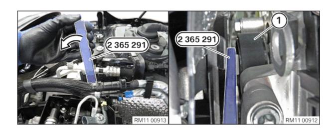
■ Designed to remove and install belt tensioners
