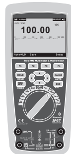
Picture 1-1 operation panel
