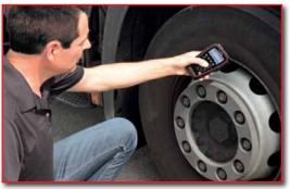
ACTIVATES AND READS ORIGINAL EQUIPMENT SENSORS IN SECONDS READS TIRE PRESSURE AND SENSOR DATA, UP TO 22 WHEELS COMPACT TO EASILY ACCESS WITHIN THE WHEEL ARCH
