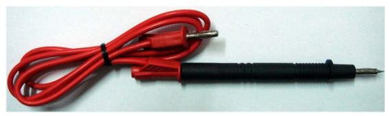
Test Probe extension with banana plug extension cable It can also be used with the banana plug extension cable to lengthen the reach of the test probes.
