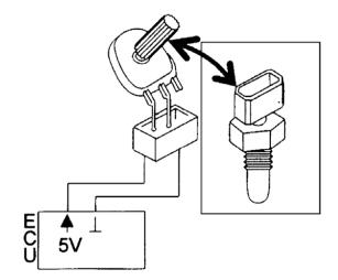
Simulating the temperature sensor signal
