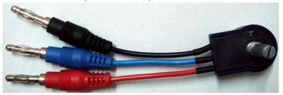
This Resistance Signal Simulator is a  $5K\Omega$  potentiometer which can simulate the resistance signals of the coolant temperature sensor, throttle valve sensor, etc.
