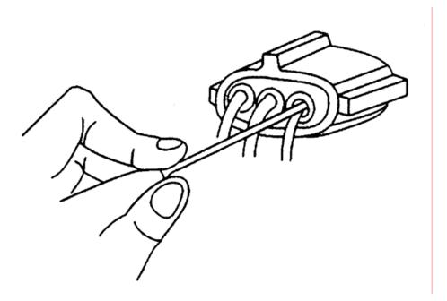
Needle probe used at the sensor connector end Caution:
