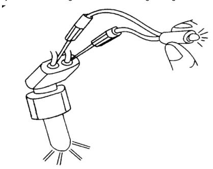
Detecting the injection pulse signal
