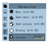
Press " ▲ " and " ▼ " keys in navigation key to select the emissivity. Then press " SELECT" key to determine selection of the emissivity. Press " ◀ " key again to return.
