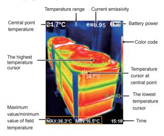
Temperature range: The range of temperature measurement.
