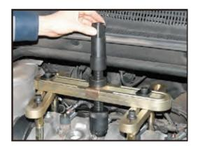
This kit is designed to remove stuck injectors from most diesel vehicles (No need to remove the electric part)
