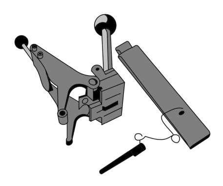
■ This tool is used to compress the valve spring for quick and safe removal / installation of the valve spring.
