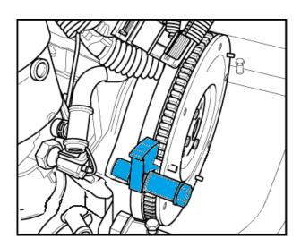
Lock flywheel when servicing clutch.
