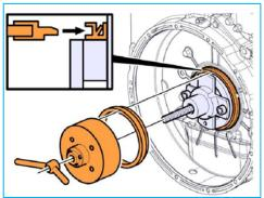
Instruction: When installing the oil seal, you won't damage the oil seal. With this tool kit will make repair be more convenient and easier.
