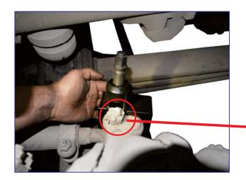
■ Put the tool onto the ball joint, you can use an air tool to turn the screw.
