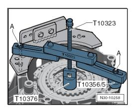
Only turn by hand. In this way, clutch slides against retaining ring.
