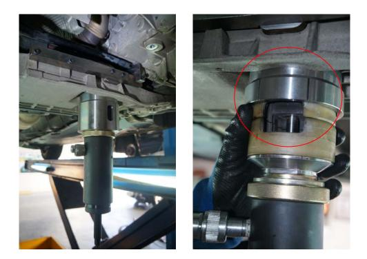
The ET1544A pulling device allows the quick and safe removal and installation of assembly carrier double-type silent blocks on the vehicle. Loosening or removing the assembly carrier from the vehicle as well as follow-up wheel alignments is not necessary.
