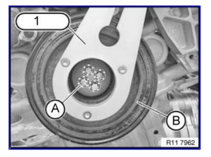
Loosen bolts (A) on the vibration absorber (B).
