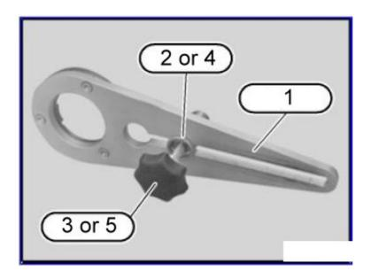
Screw A1540-1 with special tool A1540-5 into receptacle of the guide pulley.
