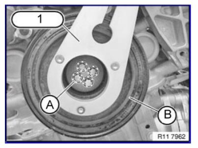
Loose bolts (A) on vibration damper (B).
