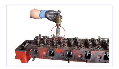
Finish removing the copper sleeve!
