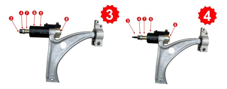
6. Attach parts no. 3. 4. 7 while the end of part no. 3 must be locked into part no. 8
