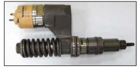
VOLVO Truck Fuel Injector Pump NUMBER: 3169521
