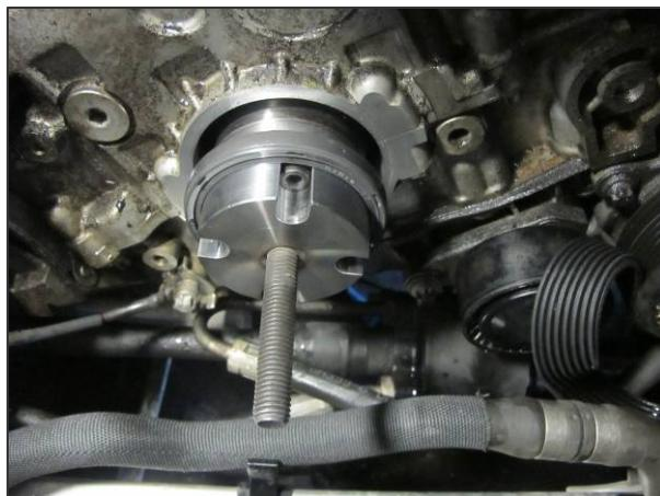
Used to loosen the seal for removal & installation of new front crank seals on BMW N52 & N54 engines. OEM Equiv: BMW 11 0 370, 11 9 220 & 11 9 230.
