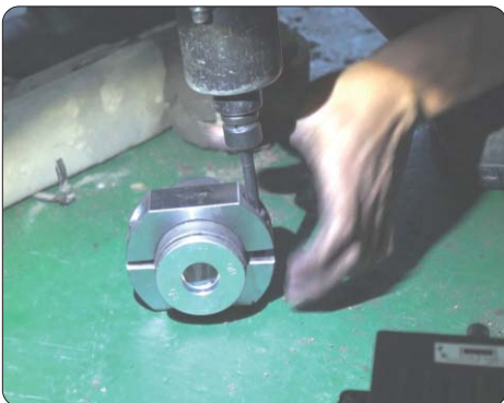
Installation of the lug pin.
