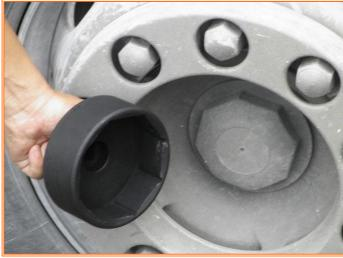
■ To dismantle the front / rear wheel axle cover of VOLVO / SCANIA trucks
