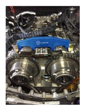
When you remove the front gear of camshaft, you must use a 32 mm wrench to hold it. Then you can use T100 socket to remove the front gear wheel.
