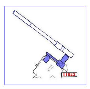
Used to hold the pinion flange for the removal / installation of the securing nut.
