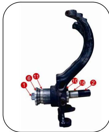
VW A4 Bearing Installation
