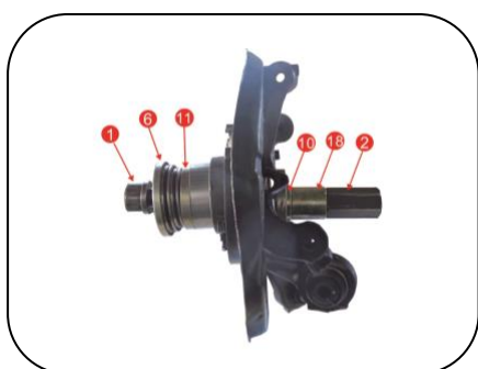
BMW E90 Bearing Installation
