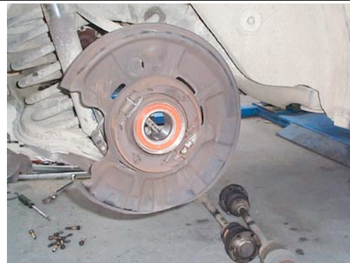
BEARING INSTALL COMPLETE
