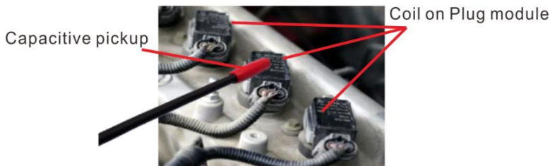
Fig. 4-Capacitive pickup on coil on plug module
