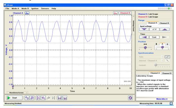
Fig.8 Output Waveform of Oxygen Sensor Zirconia
