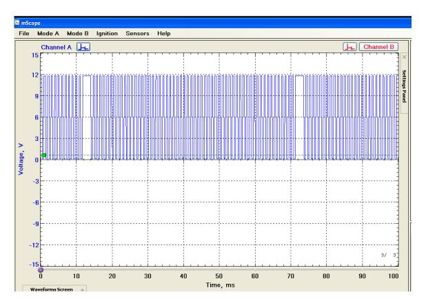
Fig.13 Output Waveform of CKP Hall Sensor
