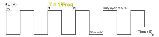
Interval of time in which some event repeats is called period. In the SI system the period is marked with T and it is measured in seconds [s]. The period T is inversely proportional to the frequency and the formula for calculation is T=1/f.
