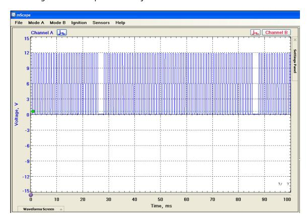
Fig.12 Output Waveform of CKP Inductive Sensor
