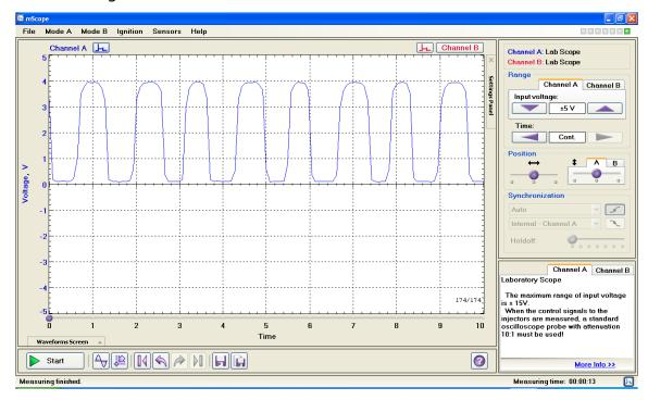
Fig.10 Output Waveform of Oxygen Sensor Titania
