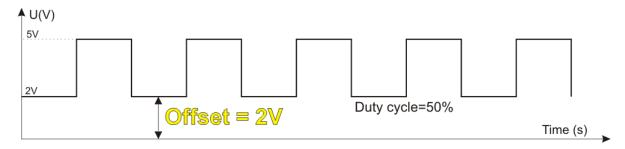
During the simulation of the signal from O2 sensor it is necessary DC offset to be used.
