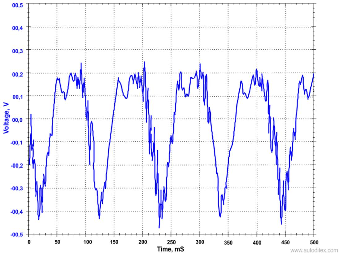
Fig.6. Exhaust gases pulsation signal Toyota Rav4. Engine is cranking (engine not started)
