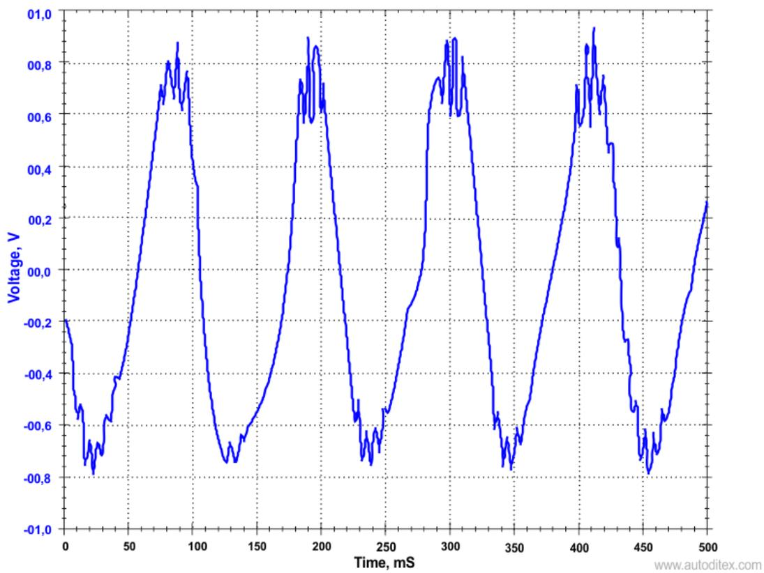
Fig.7. Intake manifold pulsation signal Toyota Rav4. Engine is cranking (engine not started)
