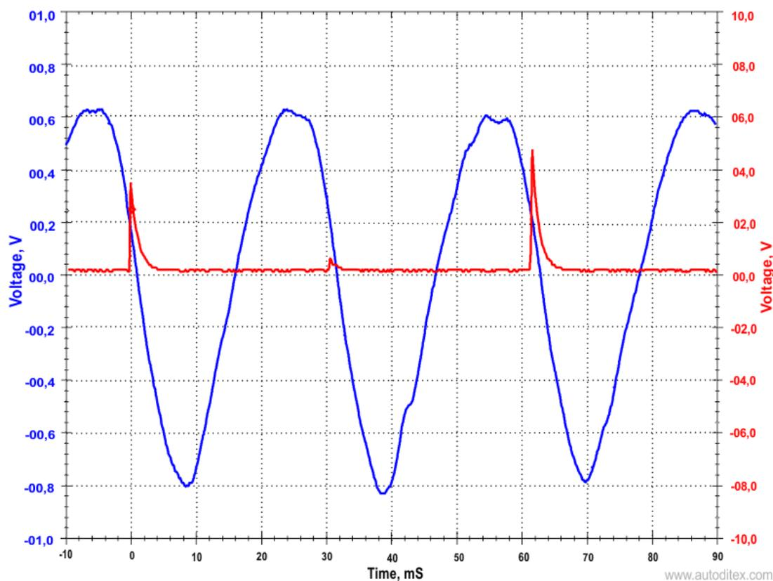
Fig.9. Exhaust pulses and 1<sup>st</sup> cylinder sync signal, 1997 Opel Astra F 1.8 16V, DIS ignition
