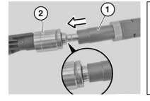
To bring the widened PTFE sealing ring to installation size, push special tool (1) as far as it will go onto injector (2). Do not use any lubricating agents.
