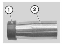
Slide new PTFE sealing ring (1) onto mounting taper (2)
