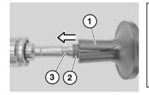
Using special tool push PTFE sealing ring into injector groove (3).
