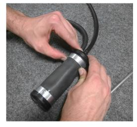
Slide Retention rings toward end of bladder, making sure bladder is centered and not twisted.
