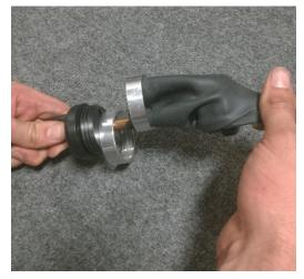
Pull bladder to be removed towards center, releasing retention rings.
