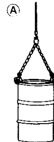
Using two clamps (This is safe when lifting a heavy drum, containing, for example, iron powder.)
